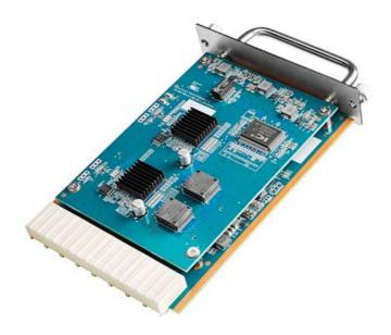
Enables an extra two channels of video output for CS200T cropping box.
