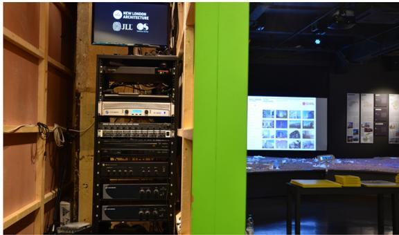
The tvONE CORIOmaster Mini video wall processor provides eight outputs connected to the projectors to create the video scaling and the edge blend and create one, large, seamless image. Using tvONE CORIOgrapher software, the individual image projected by each projector can be easily aligned. The brightness and the gamma in each of the crossover areas are adjusted to match the surrounding image perfectly.
