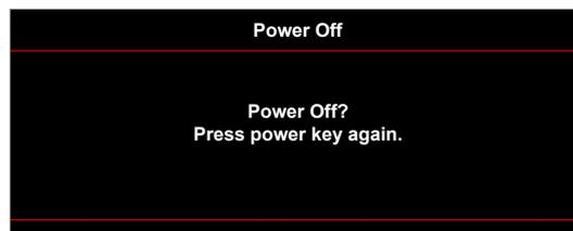
3. Press the "⏻" or the "⏻" button again to confirm, otherwise the message will disappear after 15 seconds. When you press the "⏻" or the "⏻" button for the second time, the projector will shut down.
