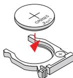
Remove the old battery and install new one (CR2025). Ensure that the side with a "+" is facing up.
